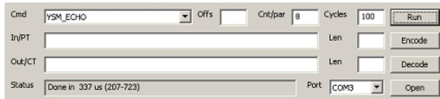
In this example, 8 bytes (Cnt/par field) are sent to the YubiHSM and echoed back 100 times (Cycles field). The average roundtrip time is 337  $\mu$ s, varying between 207 and 723  $\mu$ s.
